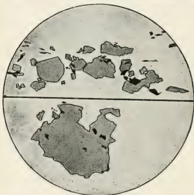
Fig. 70. Thin sections of ore from Omaha mine, Grass Valley, California. Magnified 17 diameters. Light areas, quartz; shaded areas, pyrite; black areas, gold. After W. Lindgren.*
